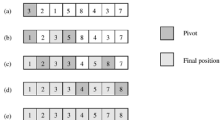
Figure 9.15. Example of the quicksort algorithm sorting a sequence of size n = 8 .
